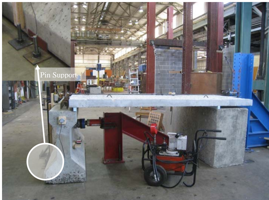
Figure 3.20 Test Setup for Girder and Deck Panel System
